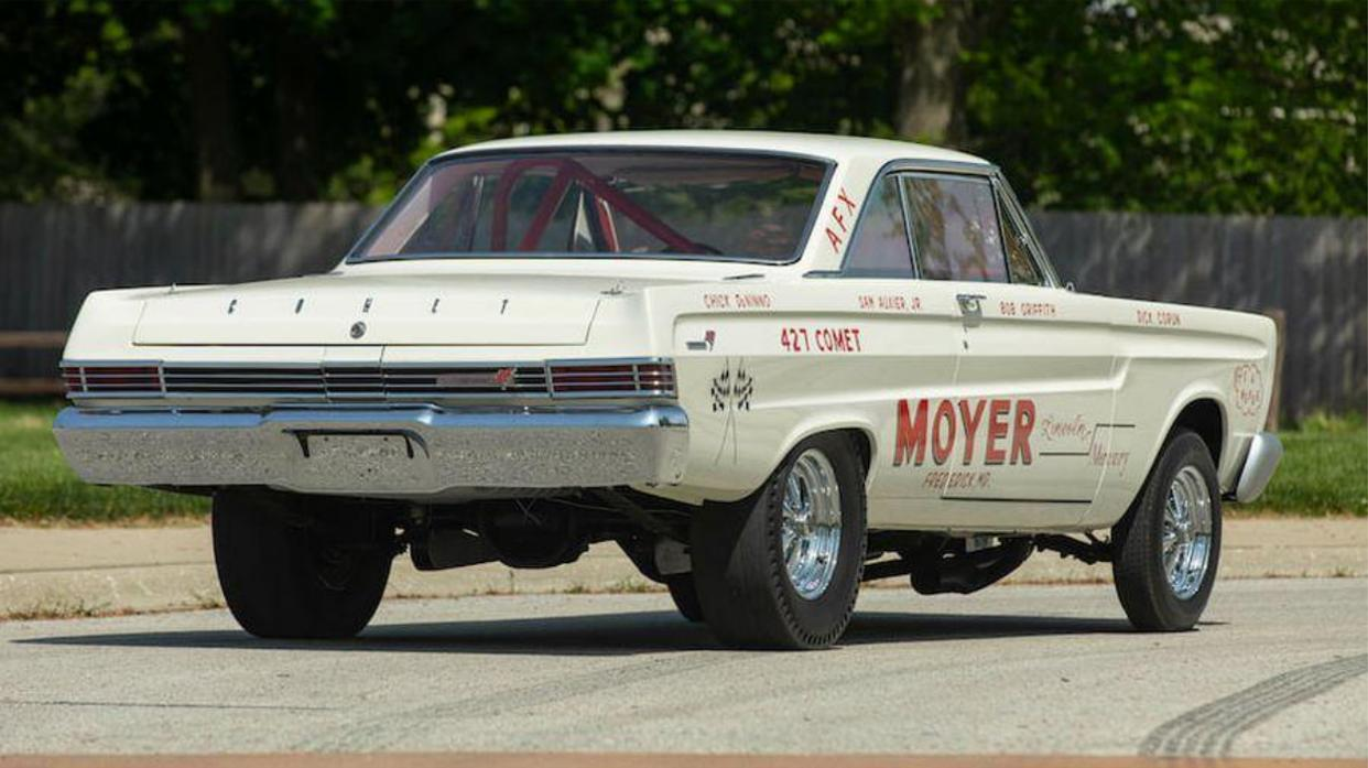
The chassis was strengthened and fitted with ladder bars and coil over shocks front and rear. The Comet wears reproduction pie crust slicks mounted on vintage re-chromed Cragar S/S mag wheels. Elapsed times were in the low 11.0-second range.
