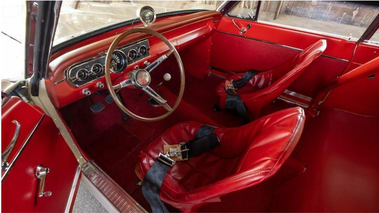
The interior is all 1960s, with low back bucket seats covered in deep red vinyl and vintage aircraft belts secure the driver for quarter-mile blasts. There's a 3-point roll bar residing between the seats for a little more head protection. The rear seat has been deleted to save weight.
