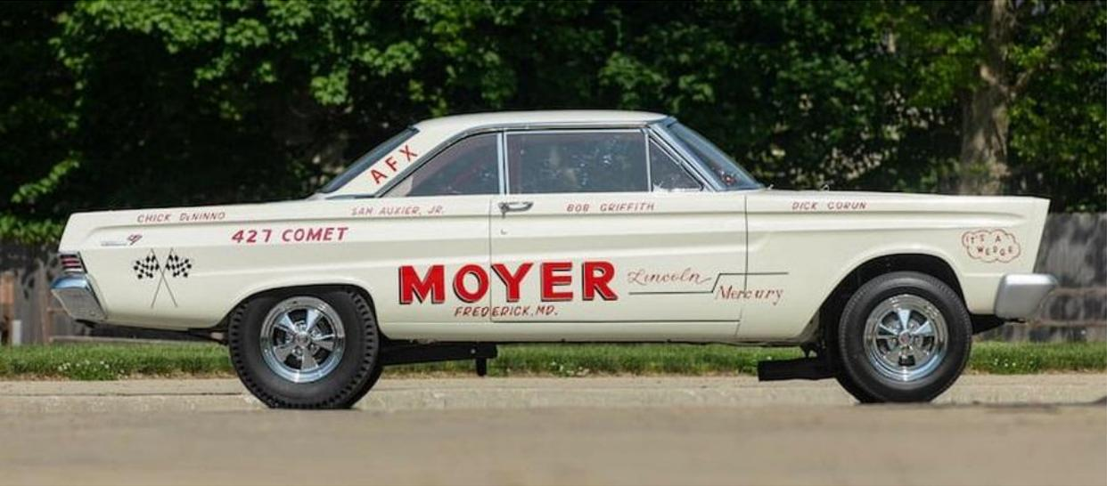
The body features lightweight fiberglass doors, hood, and bumpers. The bodies were acid dipped to save weight back in the day, and they used aluminum bumpers to save even more. The dual scooped hood is a true ram-air system connected to an airbox that feeds the dual Holley's.
