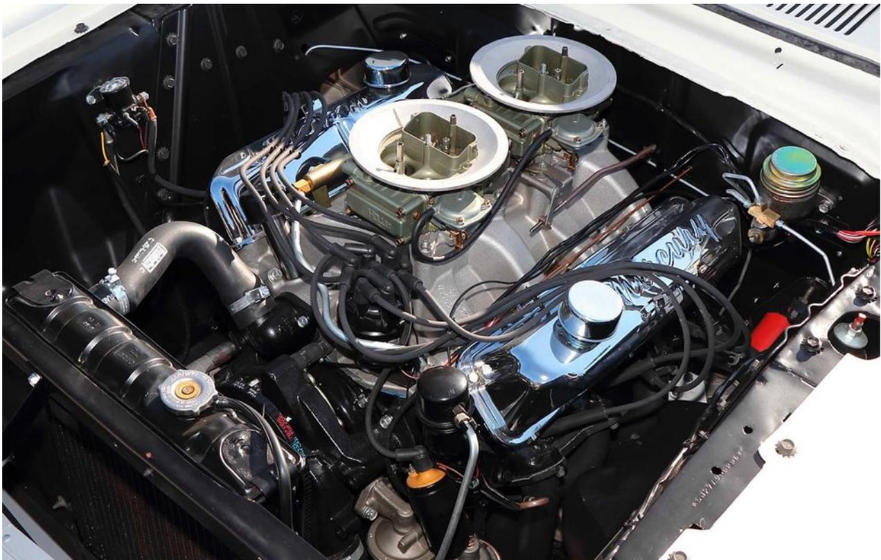
The 427 side-oiler was rebuilt with fresh internals. But the outside remains vintage-looking, not giving a clue to what's inside. The big-block features a fresh over-bore to fit a set of Ross forged pistons. The pistons are connected to a Crower billet crankshaft and Crower steel rods. The camshaft was upgraded to a roller unit, as were the rockers.
