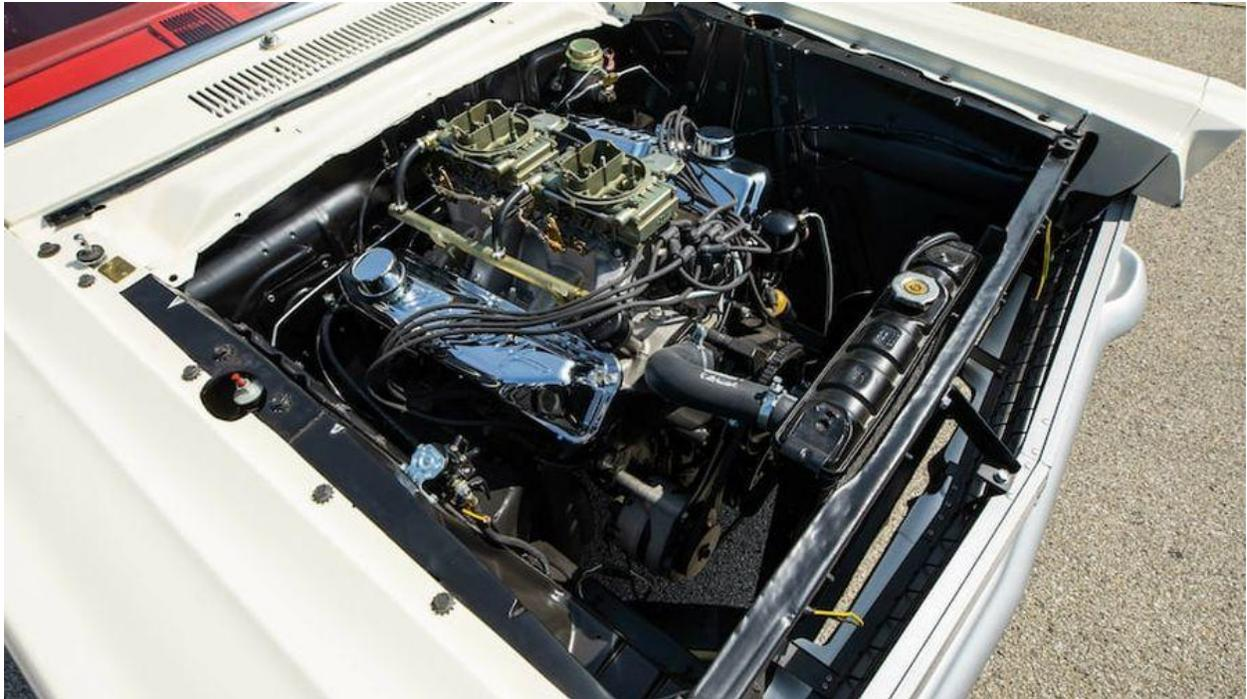
The iron heads were ported and polished by Ladd's Porting Service in Elkridge, Maryland. The Manley stainless valves and Comp valve springs and retainers keep the RPMs happy.
